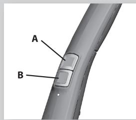
Start and stop ERGORAPIDO™ by pushing the ON/OFF button A. ERGORAPIDO™ has 2 power settings which is regulated with button B. 1. ERGORAPIDO™ will start on the high power mode. 2. For more silent cleaning and longer runtime, press the B button one more time to activate the "Silent mode".
