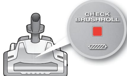
3. Brush roll indicator will be illuminated when the brush roll is overloaded. Disconnect the nozzle from tube, check status of the brushroll and clean if necessary, then re-connect.
