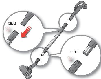
**3. Attach the telescopic tube to the floor nozzle and hose handle** (to remove them, press the lock button and pull the nozzle and hose off).
