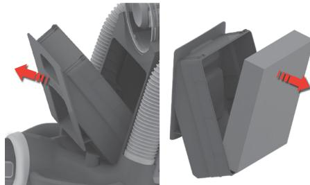
2. Remove the filter from the filter frame.
