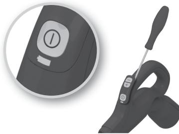
1. **Change battery when light indicator is blinking or when it is not responding when pressing any button.\***
